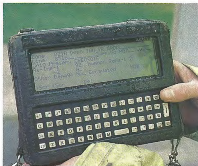
The compact Husky Hunter computer which allows the line patroller to input information to a powerful database.
